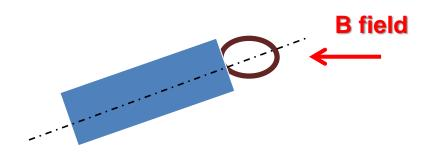
While in resonance: turn orientation of the input loop from the vertical direction in 10° steps to 360°.
