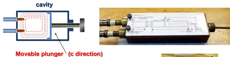
Use plunger to change the dimension of the cavity in z-direction and search for maxima in power stored using the cavity detector. Identify  $TE_{101}$  and  $TE_{102}$ .
