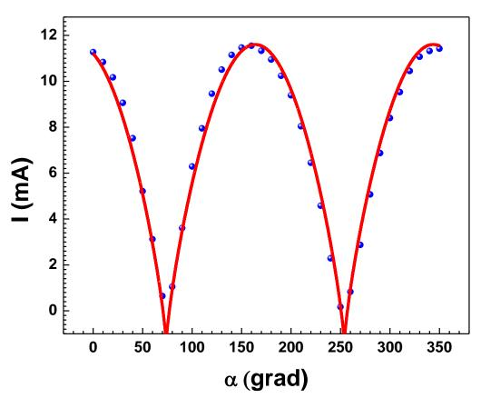
**Experimental result.** Fitted to  $A|(\cos(\alpha+\phi))^n|+A_0$
