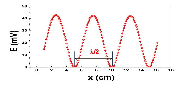
Use detector to find distance between minimums in the slotted line (wave guide). Distance between consequent minima correspond  $\lambda/2$
