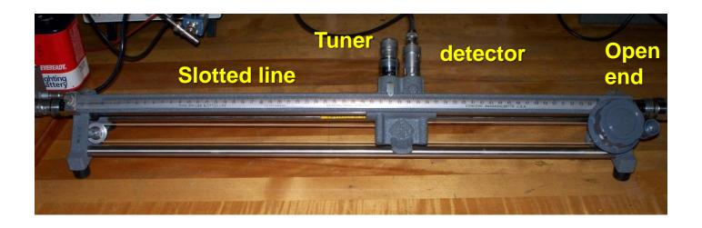
Use detector to find distance between minimums in the slotted line (wave guide)
