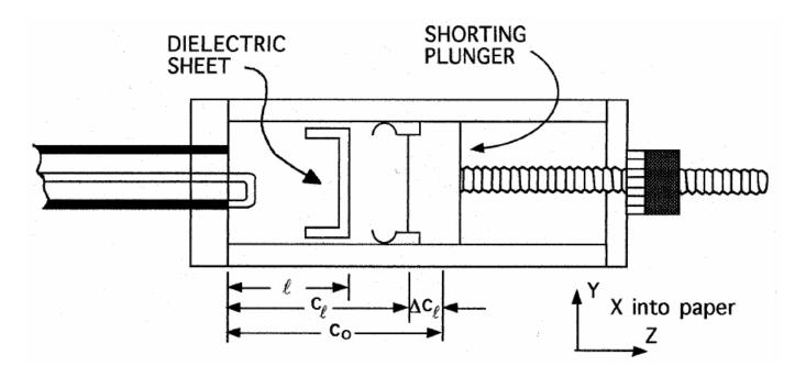
Presence of dielectric reduces length of cavity at a given resonance frequency  $\omega_0$ .
